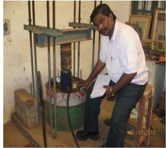
Plate 1 Author is conducting cyclic plate load tests on model flexible pavement or foundation soil bed
